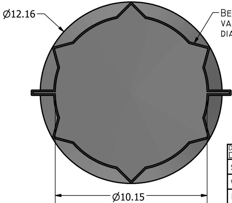
BELLOWS ALLOW FOR VARIETY OF POLE DIAMETERS
