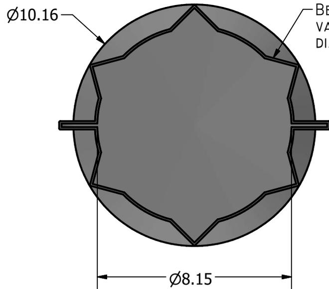
BELLOWS ALLOW FOR VARIETY OF POLE DIAMETERS
